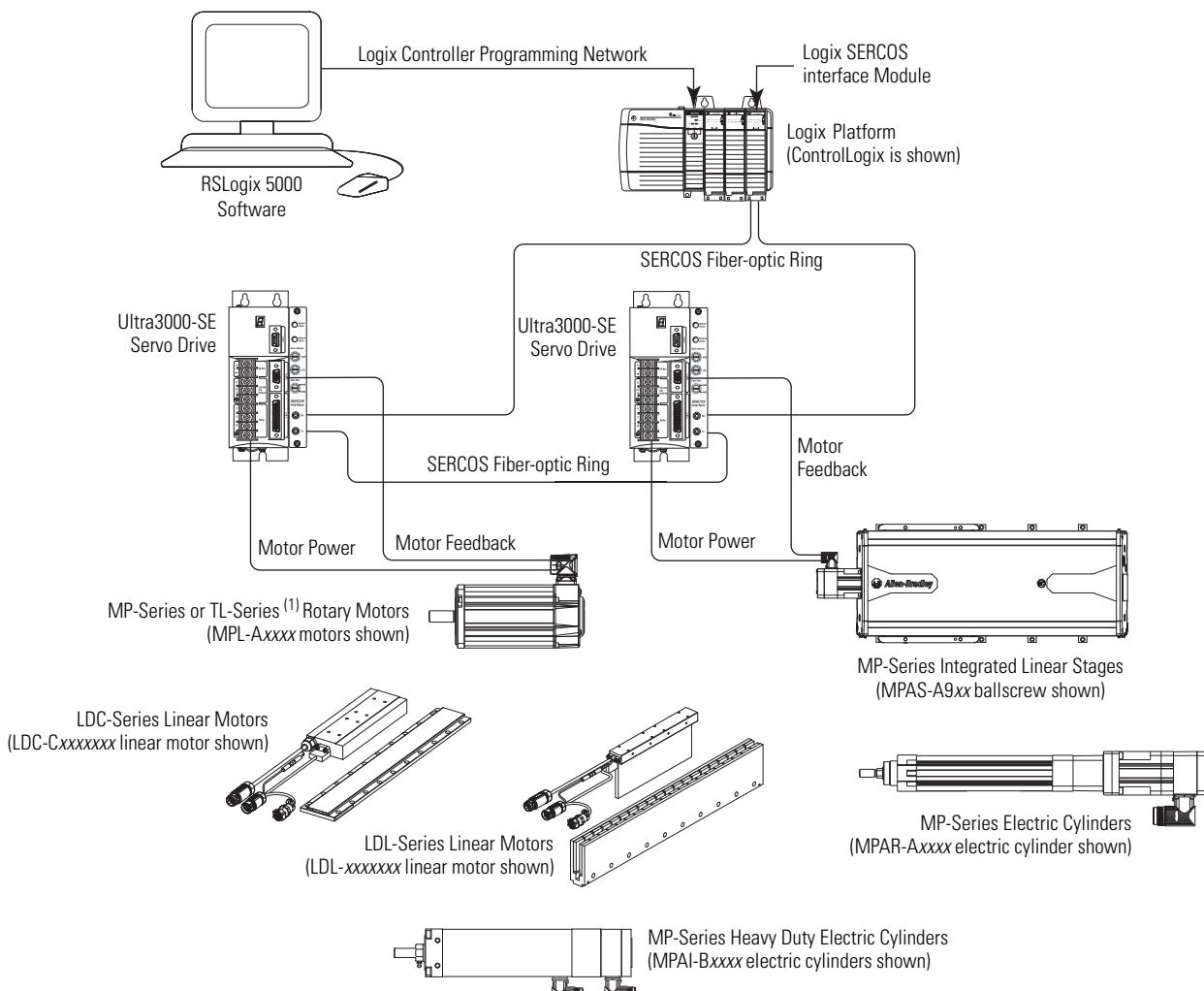
(1) Ultra3000 drives are compatible with only TL-Series (Bulletin TLY-Axxxx-H) motors with incremental encoders.
