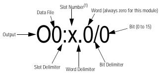
(1) I/O located on the controller (embedded I/O) is slot 0. I/O added to the controller (expansion I/O) begins with slot 1.
