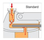
Grease Gun without TWIN-LOCK system - at high backpressure the grease flows back into the barrel (dummy-lubrication)
